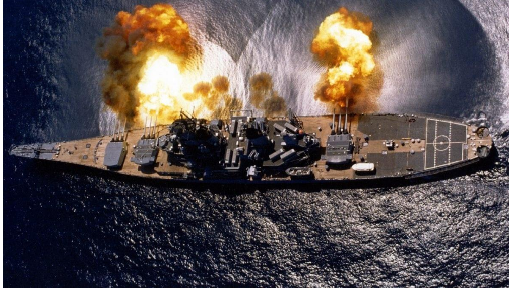
USS Iowa (BB-61) fires a full broadside of her nine 16"/50 and six 5"/38 guns during a target exercise near Vieques Island, Puerto Rico (21°N 65°W). Note concussion effects on the water surface, and 16-inch gun barrels in varying degrees of recoil.
